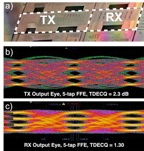
Fig. 3. a) Example 16-channel TX and RX chip. b) TX test chip output eye at 112 Gbps PAM4. c) RX test chip output eye at 112 Gbps PAM4.
