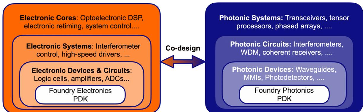
Fig. 1. Electronic-photonic design hierarchy. VLSI photonics will require the close integration and design of both disciplines.
